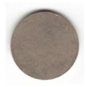
**Blanks** are the approximate size of a finished coin. They are heated in an annealing furnace to soften them, and then they are run through a washer and dryer to remove any stray grease. The shiny blanks are sorted on a riddler to screen out any that are the wrong size or incomplete shape. The clean blanks are sent through an upsetting mill, which squeezes the edges, giving them a slightly raised surface.
